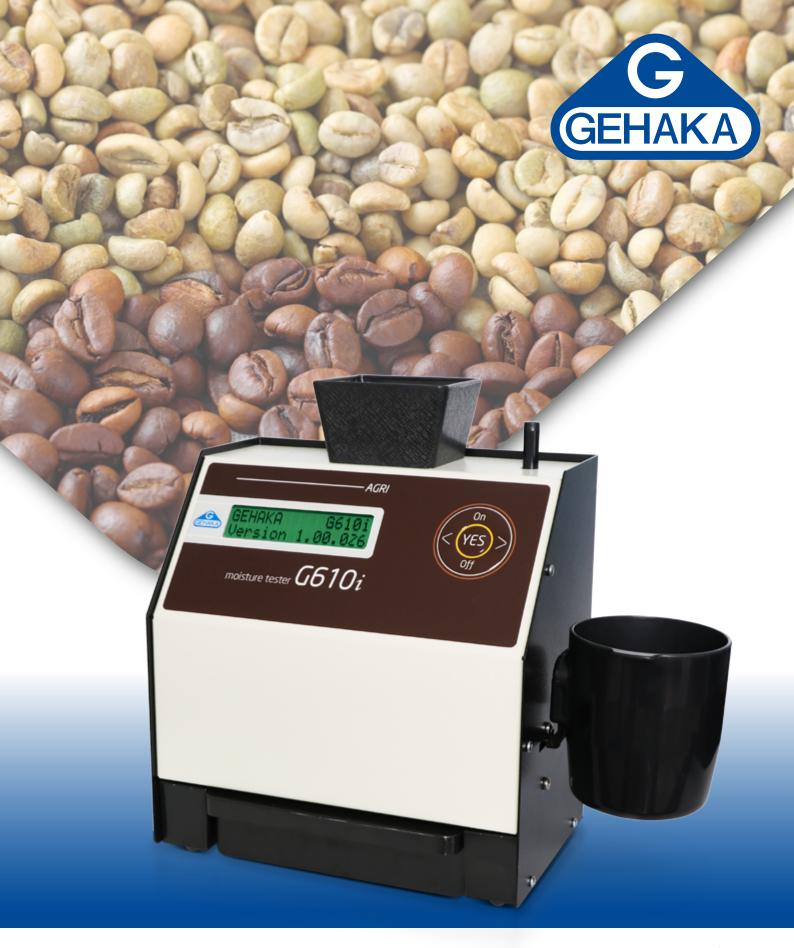
Portable grain moisture meter **G610***i*
