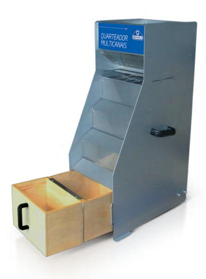
4:1 Splitter, reduces the initial sample volume to 1/4 (25%).
